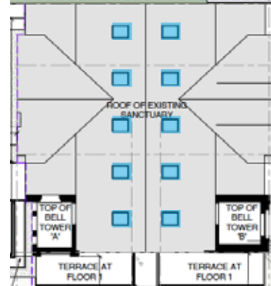
77. Proposed skylights highlighted in blue (Turner Fleischer Architects, highlighted by ERA Architects).
